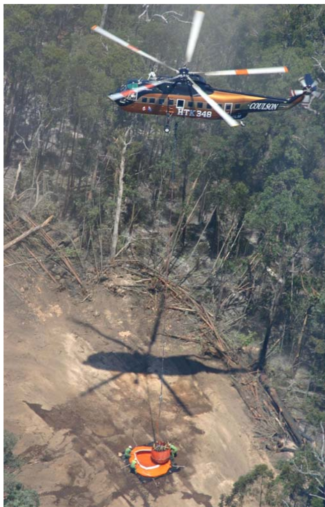
Helitack 348, a Sikorsky S61, inserting a floating collar tank at Mt Victoria, January 2008
