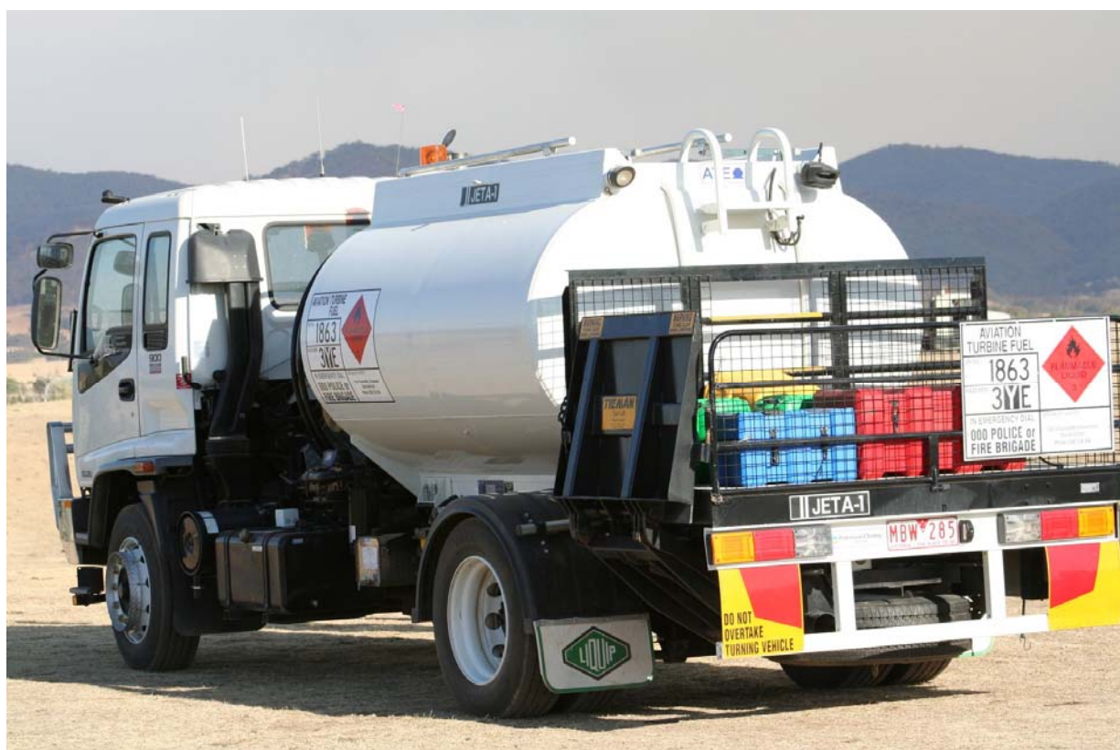
One of the five 6,000lt Jet A1 bulk refuelling tankers located across the state
